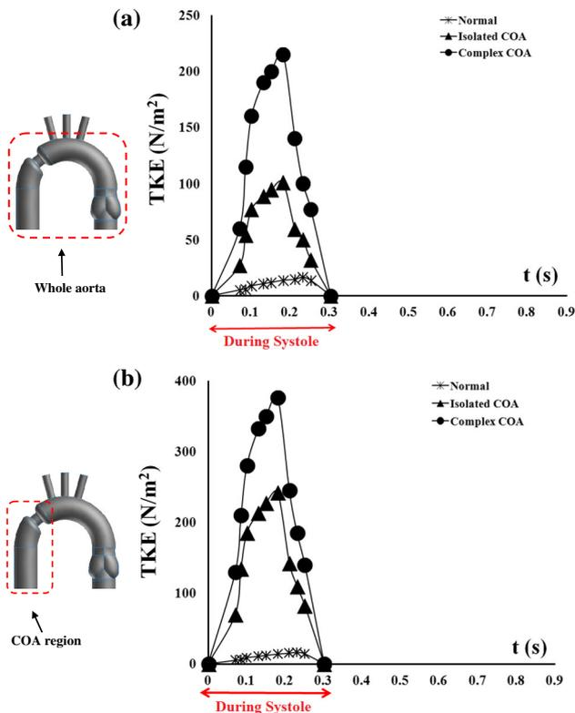
**Fig. 8** Average turbulence kinetic energy as a function of time with total flow rate of 5 L/min, **a** the averaging was performed on (central plane of the aorta) (the entire PIV domain in Fig. 1a), **b** the averaging was performed on the COA region
