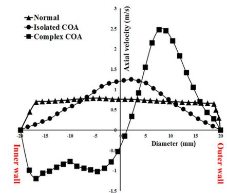
**Fig. 4** Axial velocity profiles at different sections of the aorta and at the peak of systole (*point E* in Fig. 2) with total flow rate of 5 L/min
