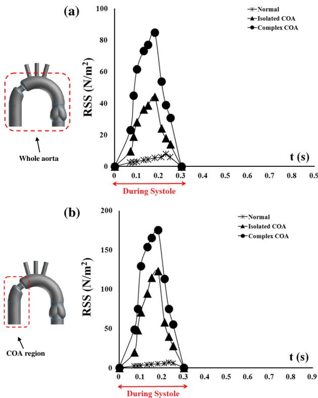
**Fig. 10** Average Reynolds shear stress as a function of time with total flow rate of 5 L/min, **a** the averaging was performed on (central plane of the aorta) (the entire PIV domain in Fig. 1a), **b** the averaging was performed on the COA region
