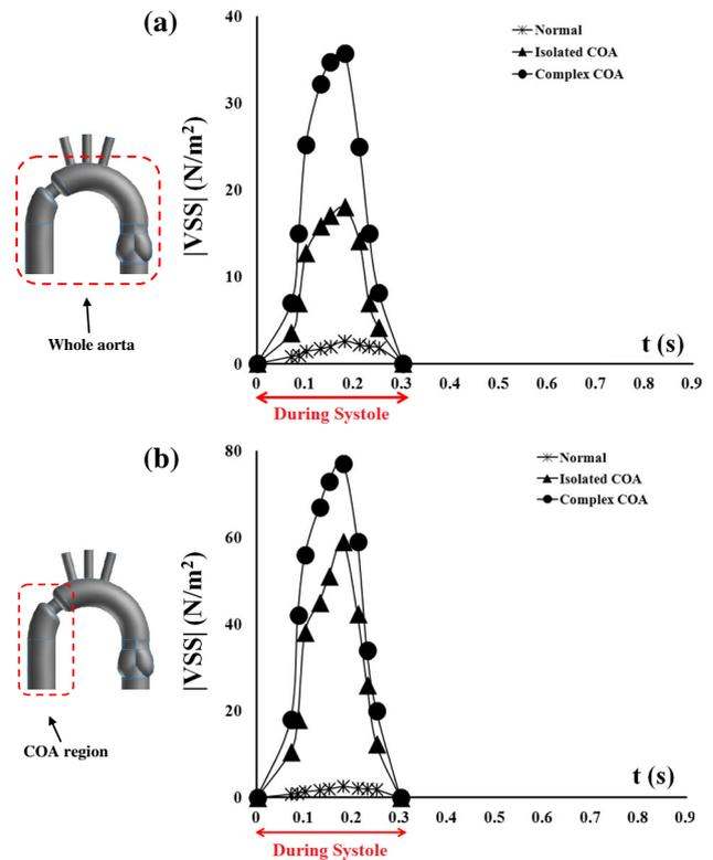
**Fig. 7** Average absolute viscous shear stress as a function of time with total flow rate of 5 L/min, **a** the averaging was performed on (central plane of the aorta) (the entire PIV domain in Fig. 1a), **b** the averaging was performed on the COA region
