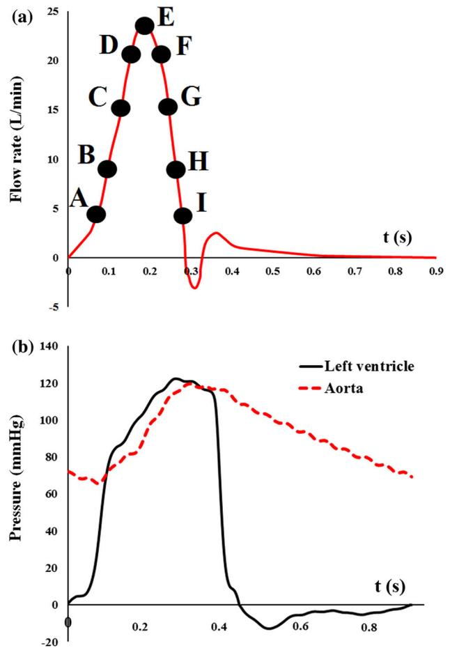
**Fig. 2** a Flow rate measured downstream of the aortic valve and time points of PIV experiments (total flow rate: 5 L/min), b unfiltered pressure wave forms obtained from in vitro model in normal condition (without COA and/or BAV) (total flow rate: 5 L/min)
